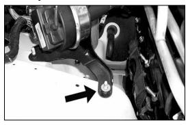
18. Install the provided ¼ washer onto existing nut that retains the cruise control bracket to vehicle.
