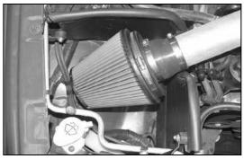
39. Install the air filter assembly onto the intake tube and secure with the provided hose clamp. NOTE: Drycharger® air filter wrap; part # RF-1048DK is available to purchase separately. To learn more about Drycharger® filter wraps or look up color availability please visit http://www.knfilters.com®.
