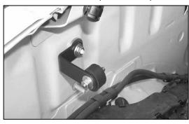
13. On vehicles that did not come with a TCM, mount "L" bracket onto existing stud with the provided hardware.
