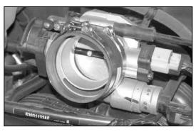
23. Install the silicone hose (084031) onto the throttle body with supplied hose clamps.
