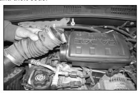
2. On vehicles with an intake resonator, loosen the hose clamp at the resonator and remove the intake hose as shown.
