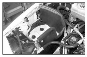
20. Install heat shield onto the vehicle with the provided hardware as shown.
