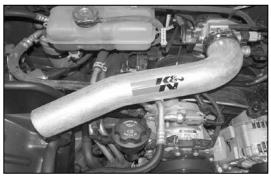
24. Install the K&N® intake tube into the silicone hose at the throttle body and align with the mounting bracket installed in step #22.
