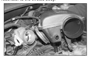
9. Pull firmly to dislodge the resonator from the mounting grommets and remove the resonator from the vehicle.
