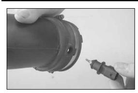
28. Remove the air temperature sensor from the stock intake tube as shown.
