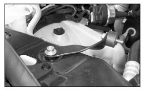
16. Install the bracket onto core support with the provided allen bolt as shown.
