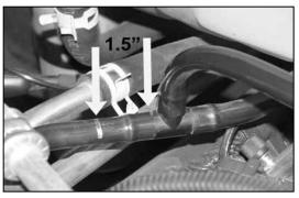
30. On vehicles equipped with the intake resonator, measure 1.5" from the crank case vent hose "T' and cut the crank case vent tube with knife.
