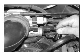
4. On vehicles equipped with an intake air temperature sensor, disconnect the electrical connection from the air temperature sensor as shown
