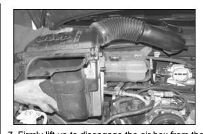
7. Firmly lift up to disengage the air box from the mounting grommets and remove the air box from the vehicle.
