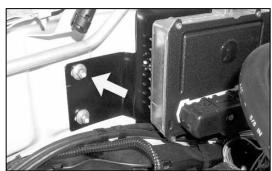
11. Remove nut from inner fender on vehicles that come equipped with a TCM.
