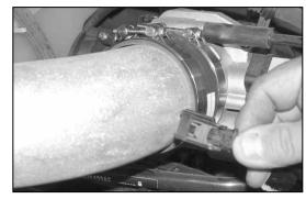
25. On vehicles equipped with an air temperature sensor, position the temperature sensor electrical connection for best fit and mark the location to be drilled. Remove the K&N® intake tube.
