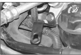
22. Using the bolt removed in step #21, install the tube mounting bracket (010064) onto the A/C pump as shown.
