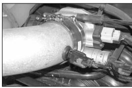
35. On vehicles equipped with the air temperature sensor, reconnect the sensor electrical connection.
