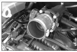
23a. On 2007 and later vehicles with a plastic throttle body, install the silicone hose (08096) onto the throttle body and secure with the provided hose clamp.
