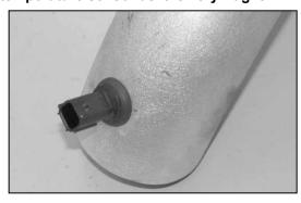
29. Install the air temperature sensor into the grommet in the K&N® intake tube as shown.
