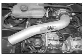
34. Reinstall the K&N® intake tube and secure with the provided hardware.
