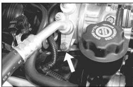
21. Remove the A/C compressor-mounting bolt.
