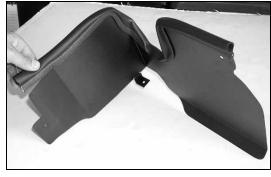
17. Install edge trim onto heat shield as shown. NOTE: Some trimming of the edge trim will be necessary.
