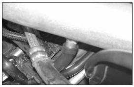
36. Connect the supplied crank case vent hose onto the K&N® intake tube.
