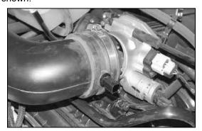
5. On vehicles not equipped with a intake resonator, loosen the hose clamp which secures the intake tube to the throttle body and then disconnect the intake tube from the throttle body as shown.
