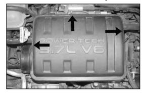
8. On vehicles equipped with an intake resonator, disconnect the two crank case vent hose shown and loosen the hose clamp, which secures the resonator to the throttle body.
